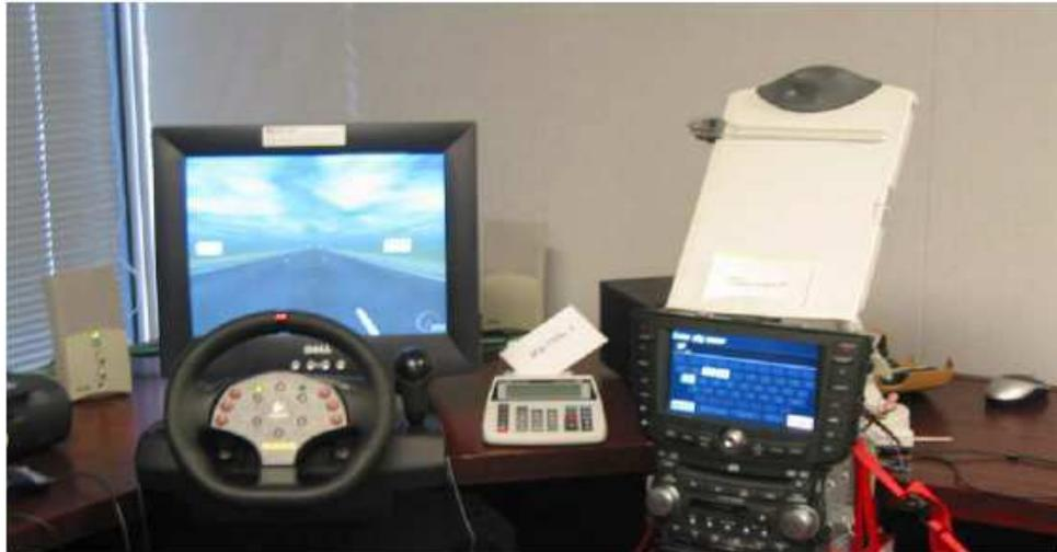
Figure 3.3 Lane-change task set-up (from Burns, 2006, used with permission)
