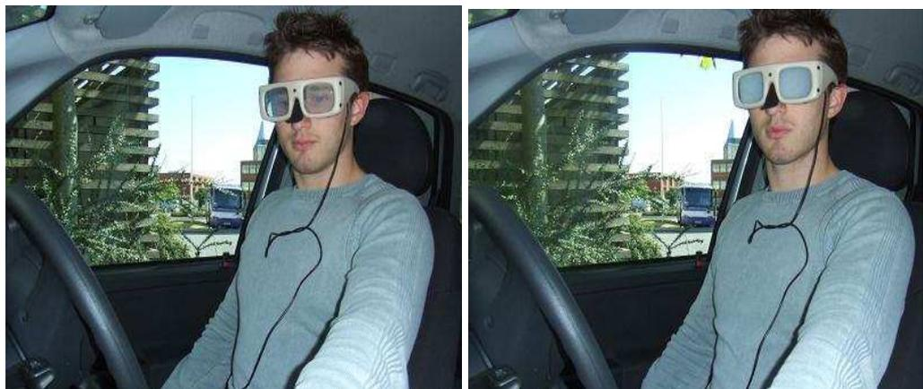
**Figure 3.2 Occlusion goggles: (a) shutters open; (b) shutters closed**
