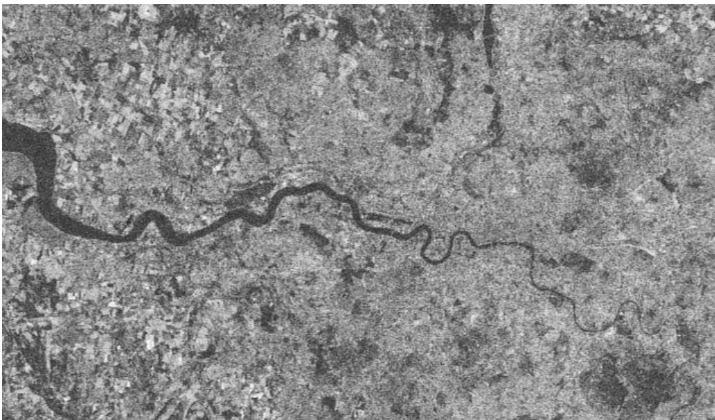
Figure 3.5. An example of a coherence image: corresponding to interferograms from Figs. 3.3 and 3.4; the river Thames can be easily identified from this image.
