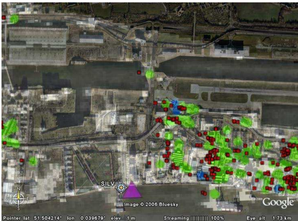
Figure 8.8 Greenwich: Aerial image with PS points overlain (of the London Docklands region). Red squares denote PS points as geocoded onto the aerial image, green and blue circles denote corrected PS location using the radar image.
