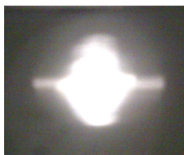
Figure 4.7: Picture of the pump beam profile on entry into the SEOP oven.
