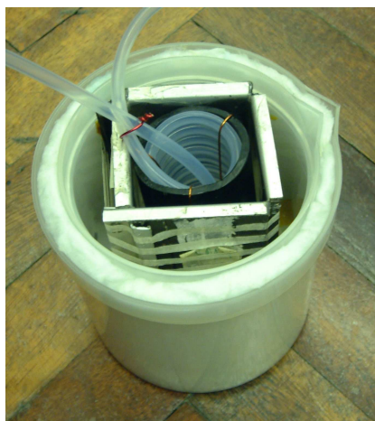
Figure 4.20: Picture of our Xe freeze out coil inside a four pole magnet and liquid nitrogen bath.
