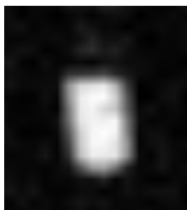
Figure 7.5: Image of ^{129}\text{Xe} dissolved in toluene in the bottom of a 60 ml syringe. The image has an SNR of 60 and it is possible to make out the conical shaped end of the syringe. There exists practically no signal from ^{129}\text{Xe} in the gas phase above the toluene.
