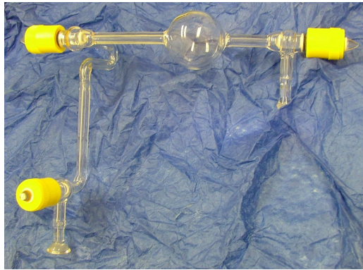
Figure 4.13: Photograph of the spherical flow cell.
