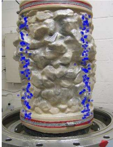
Figure 5.8. Meshes on the sample at the end of the test
