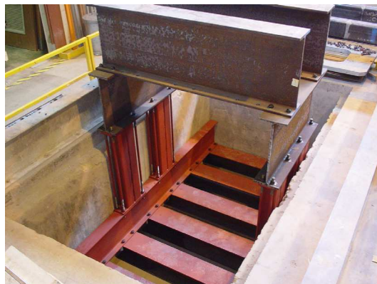
Figure 4.2. Testing frame in the pit
