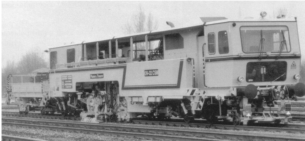
Figure 2.3. Self-propelled tamping machine (Selig and Waters, 1994)
