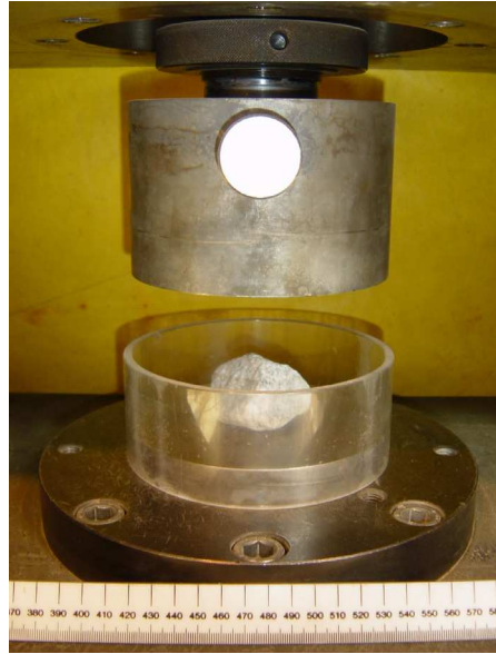
Figure 3.2. Configuration of a single particle crushing test
