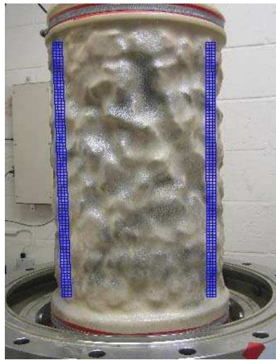
Figure 5.6. Meshes on the sample at the beginning of the test
