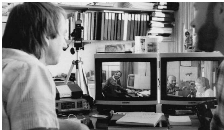
Figure 2.3 A media space (showing two connected nodes)
