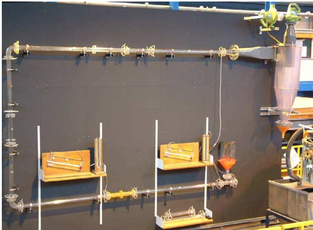
Figure 5.4: The final pneumatic conveying rig for the present study
