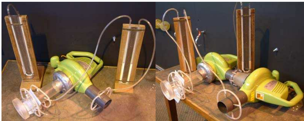
Figure 5.26: Experimental setup for fan tests
