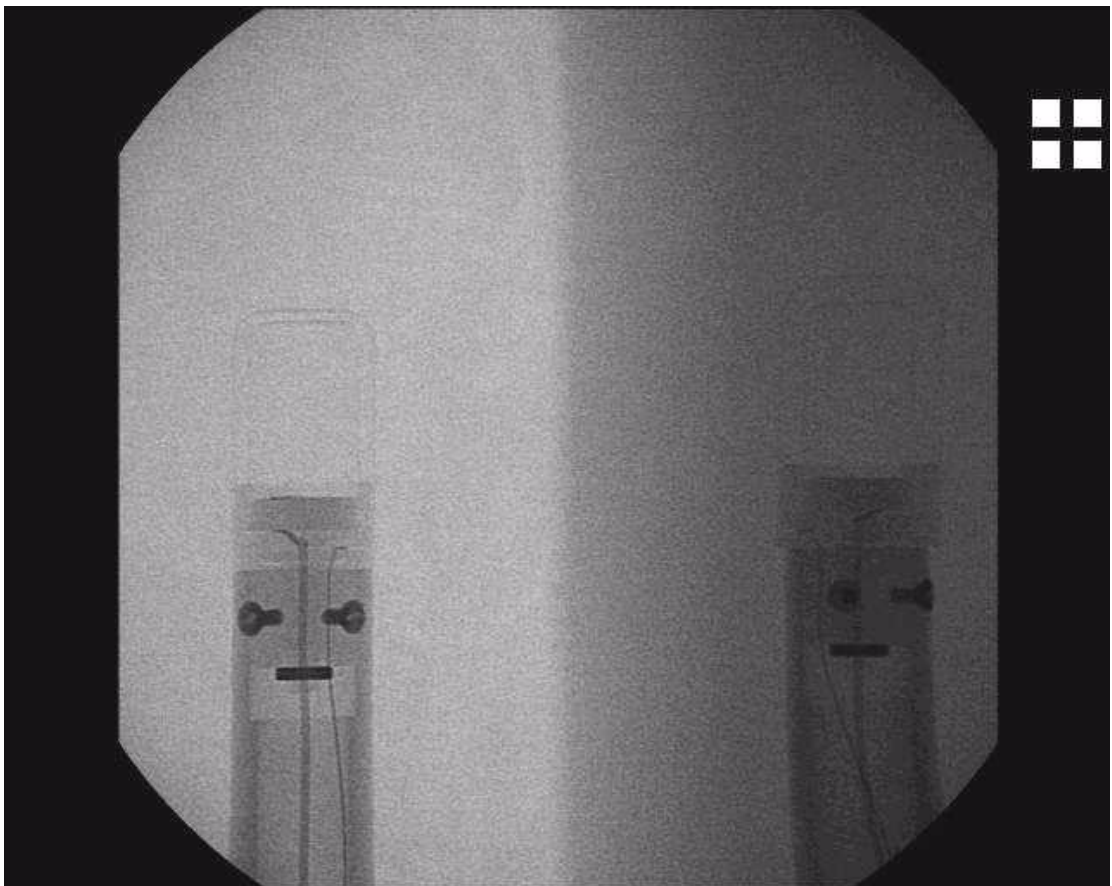
Figure 4.3: Dose meter positions for wedge filter measurements.
