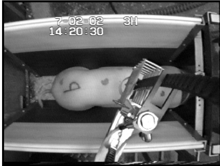
Figure 3.8 Example of how the robot arm obscures some kink points, but leaves the rump clearly visible. The rear kink features are often obscured as the robot moves.
