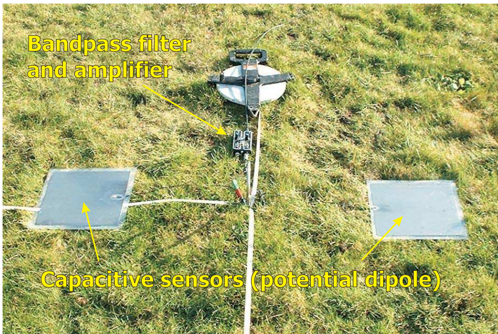
Figure 6.4: Potential dipole of the BGS prototype CRI system. ©NERC copyright.
