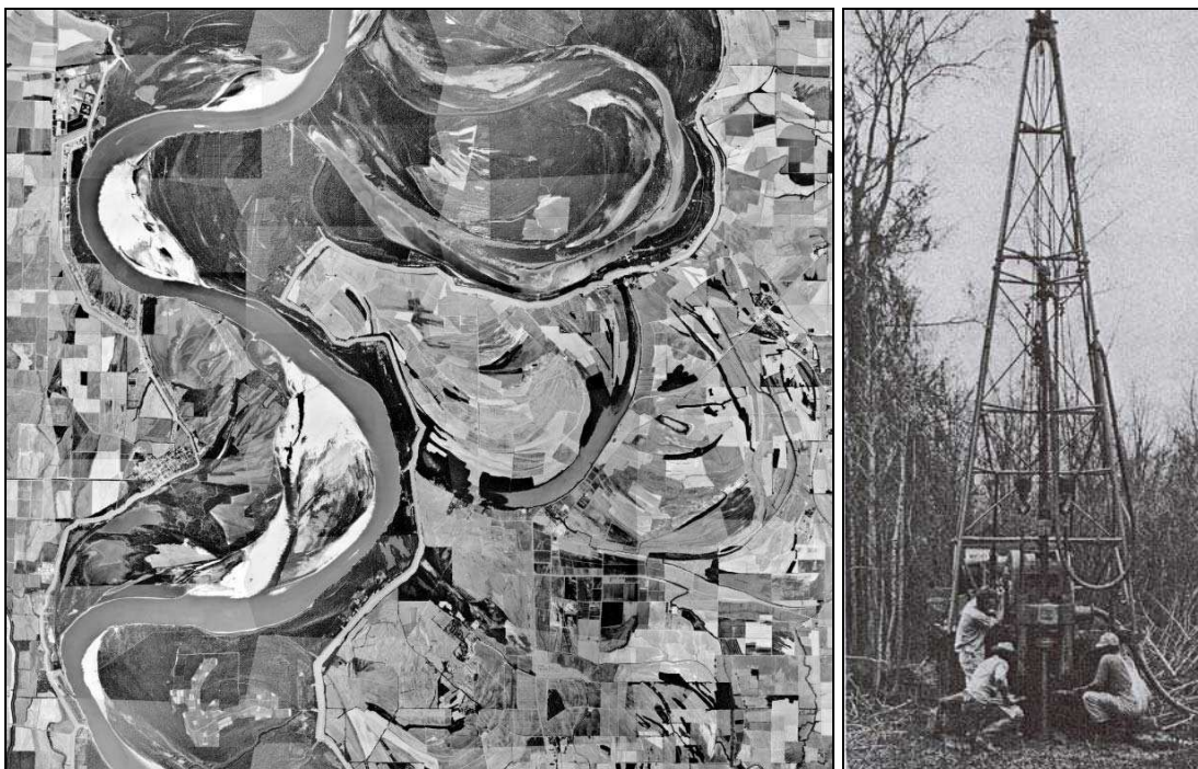
Figure 2.16 a) Aerial photograph mosaic of the ‘Cat-Fish Point’ bend reach of the Lower Mississippi River, collected by the USACE Vicksburg District in 1999 at an original scale of 1:20 000. b) A team undertaking subsurface borings in the alluvial valley (Moore, 1972).
