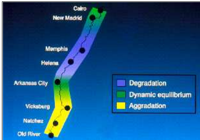
Figure 2.15 Regional-scale adjustments to the longitudinal profile in the period 1950-94, as proposed by Biedenharn and Watson (1997).
