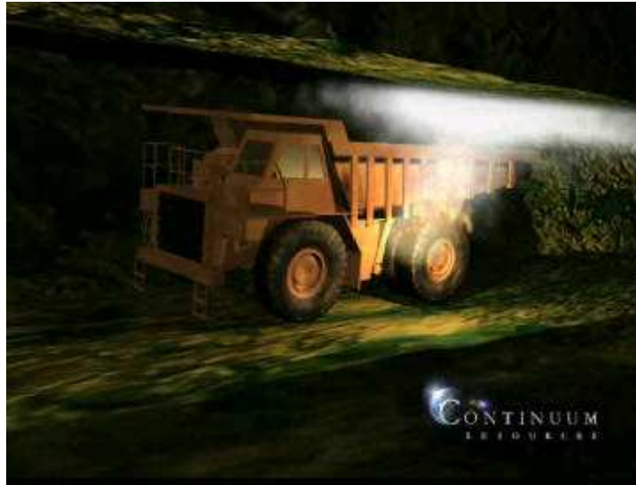
Figure 6-14: Haul truck on fire in decline
