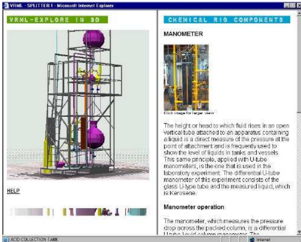
Figure 6.49: The VRML model with an explanation of manometer operation
