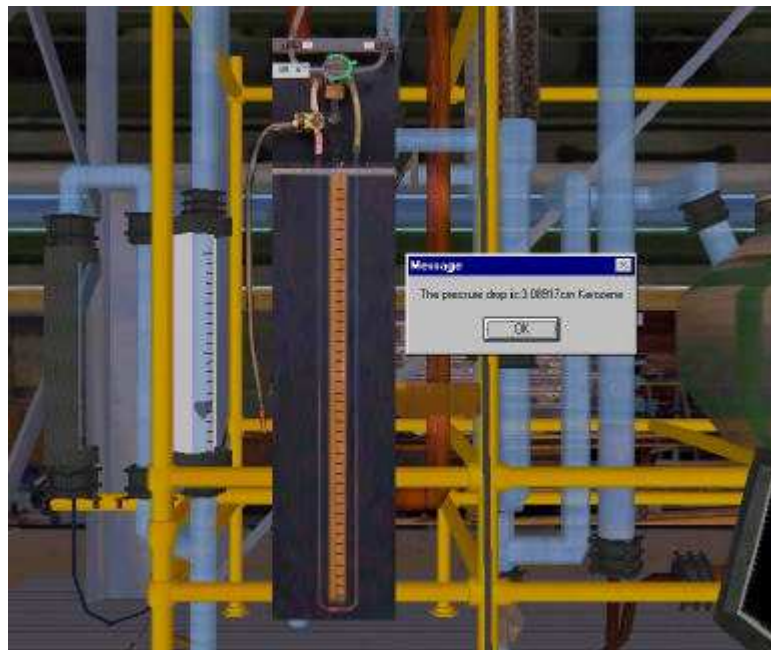
Figure 6.46: Pressure drop reading
