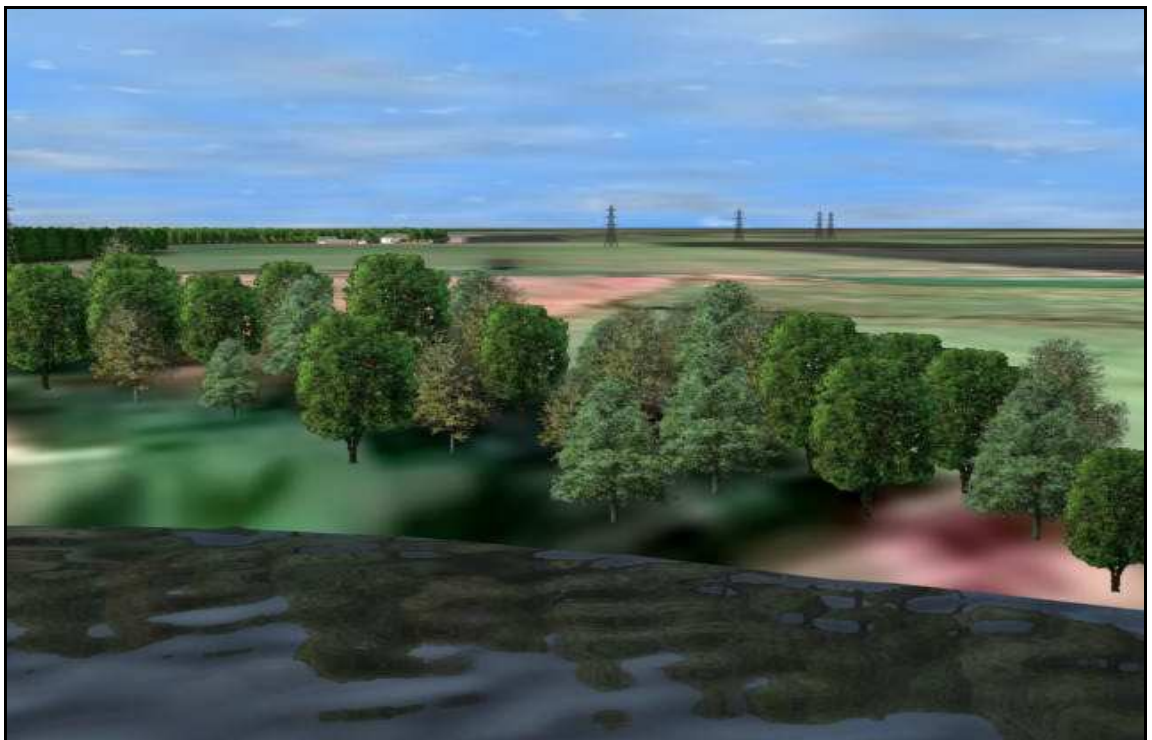
Figure 6.45: Reflection and bump map applied to an extruded spline to simulate the river 165 .
