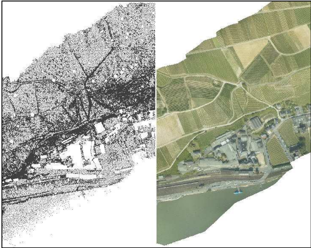
Figure 4.12: Laser scan point cloud and the ortho-rectified aerial image of the proposed site 73 .
