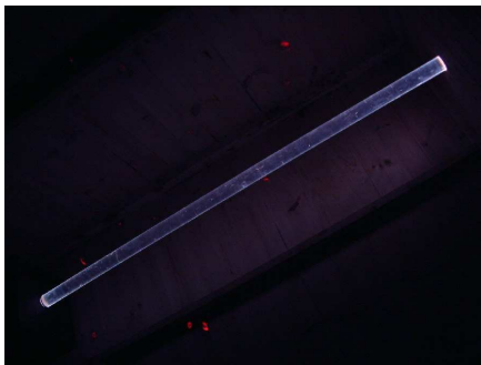
Fig. 4 - 10: Rod leakage in darkened chamber
