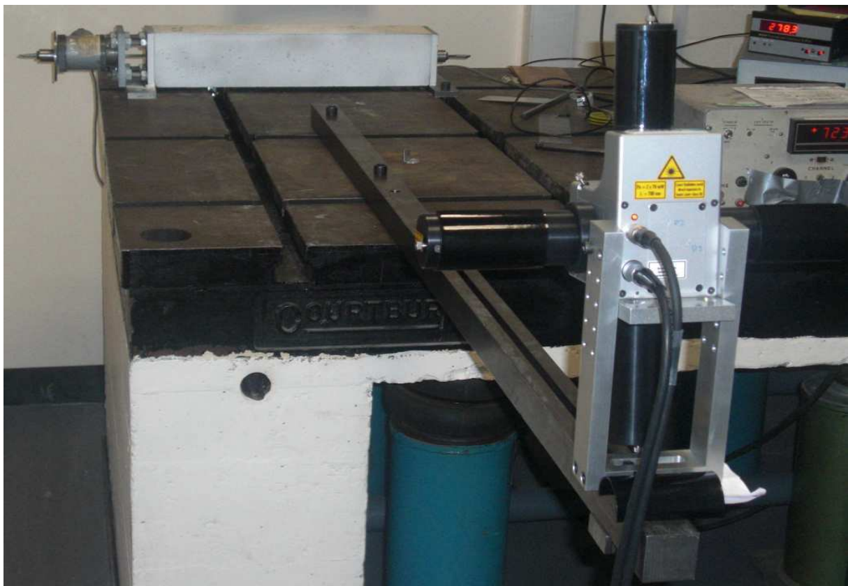
Figure 2: Test setup showing specimen and ESPI camera
