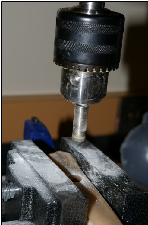
Figure 2.4: Drilling of a bone core sample for mechanical analysis.
