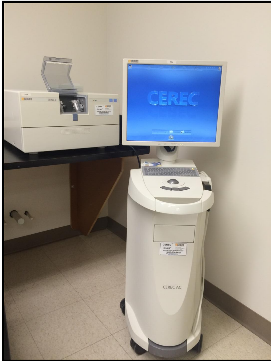
Figure 13: CEREC (Sirona) unit with Bluecam scanner and CEREC inLab (Sirona) milling unit.
