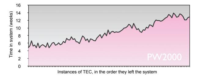
Figure 14: Steadily increasing 'time in system' is a symptom of a system with poor logistic control, where the rate at which products enter the business unit exceeds its capacity
