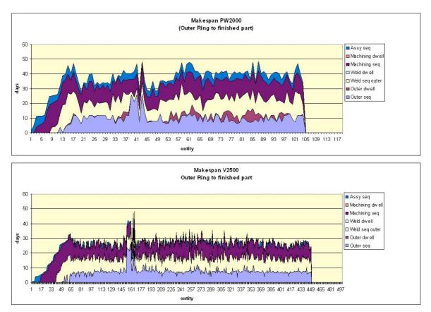
Figure 83: Lead times observed, with a machine breakdown under OPT
