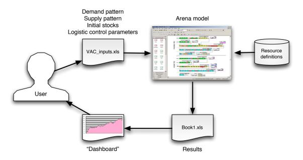
Figure 10: Logistic simulation system architecture
