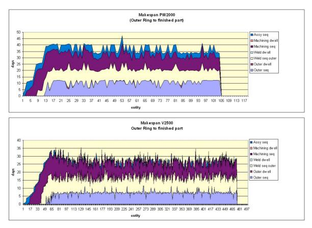
Figure 35: Lead times observed, steady state OPT system
