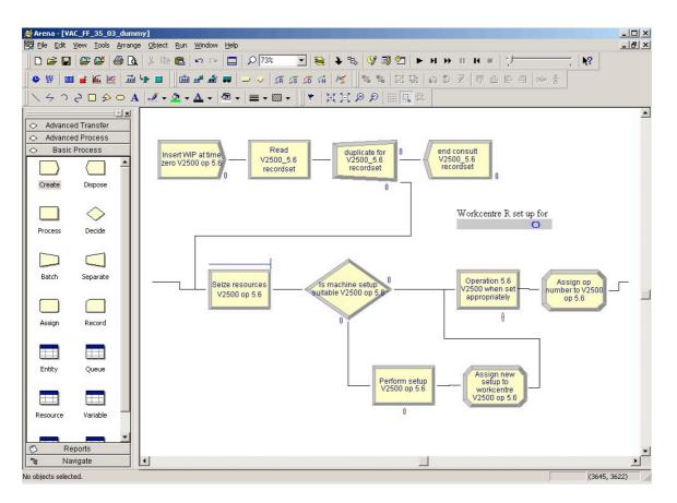
Figure 8: Focused factory submodel, including a means of populating the simulation with WIP at the start of the model run (the top four modules achieve this).
