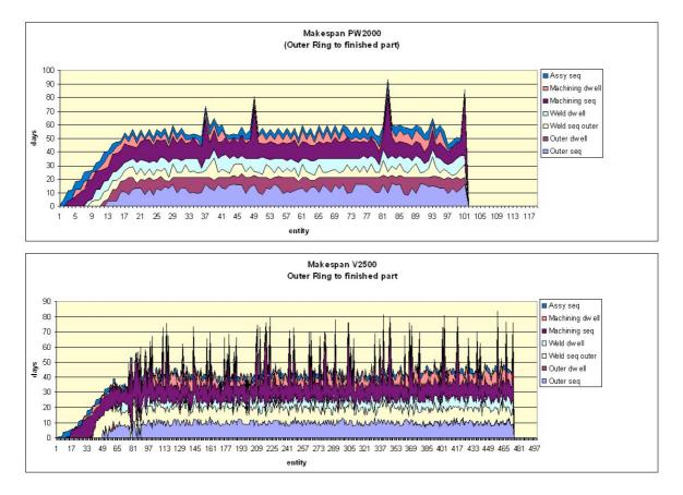
Figure 55: Lead times observed, with quality problems in a 'pull' system
