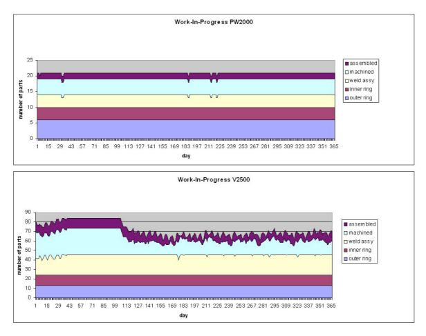
Figure 81: WIP levels observed, with a machine breakdown under a 'pull' system
