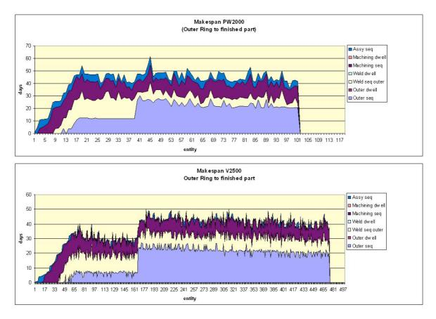
Figure 75: Lead times observed, with a machine breakdown under a 'push' system
