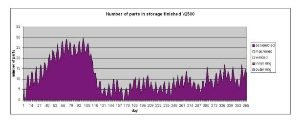
Figure 77: Stock of V2500 TECs, with a machine breakdown under a 'push' system
