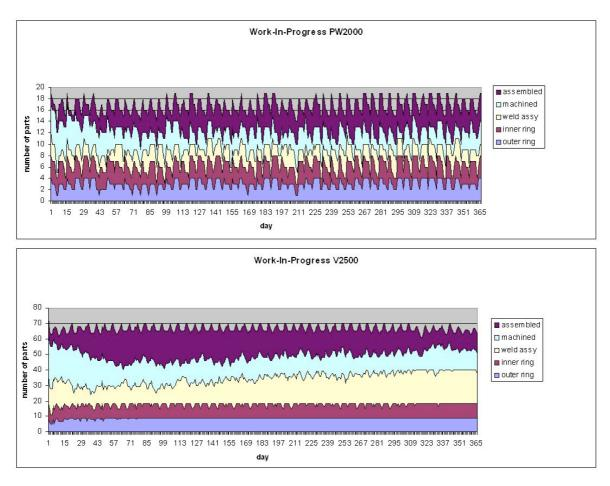
Figure 36: WIP levels observed, steady state OPT system
