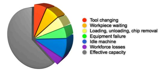
Figure 25: Losses in effective production capacity
