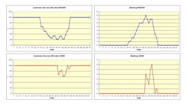
Figure 45: Fill rates achieved (and backlog), with the experimental demand pattern changes under a 'pull' system
