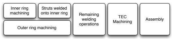
Figure 3: Basic operations sequence for TEC manufacture
