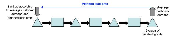
Figure 30: Application of a planned lead time in a 'push' scheduled system
