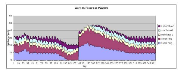
Figure 22: Sample output showing the level of WIP within the focused factory
