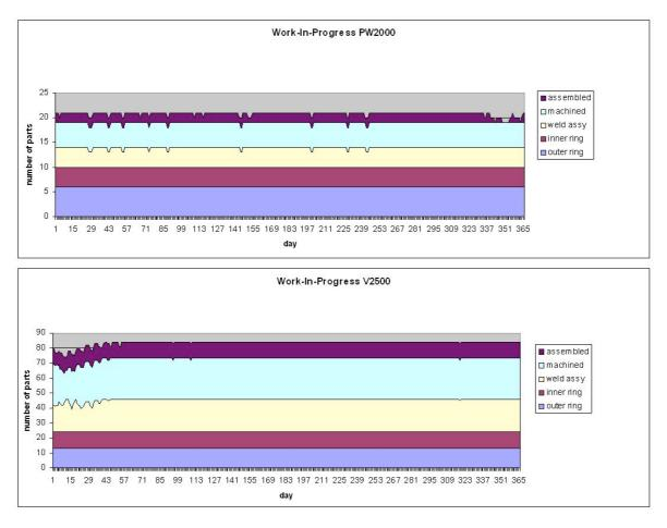
Figure 57: WIP levels observed, with quality problems under a 'pull' system
