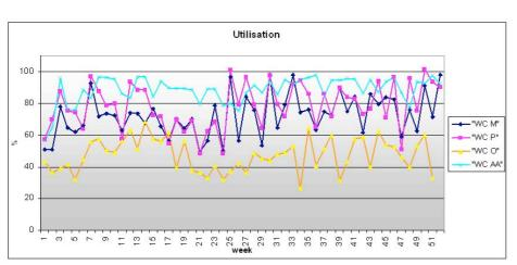
Figure 74: Observed utilisation of key workcentres, with a supply shortage under OPT
