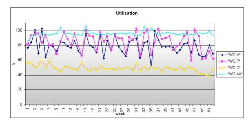
Figure 58: Observed utilisation of key workcentres, with demand pattern changes under a 'pull' system
