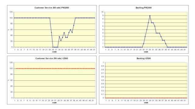
Figure 64: Fill rates and backlogs, with a supply shortage under 'pull' logistic control
