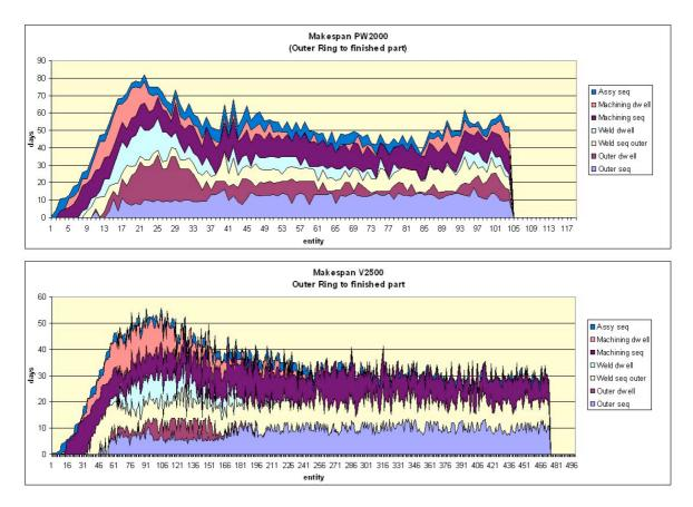
Figure 44: Lead times observed, with demand pattern changes under a 'pull' system
