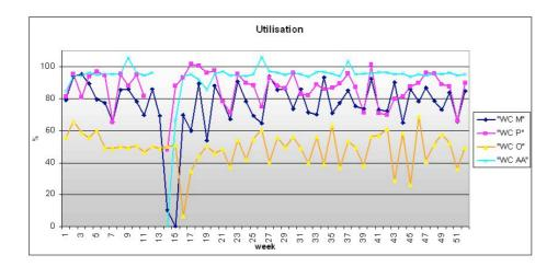
Figure 82: Observed utilisation of key workcentres, with a machine breakdown under a 'pull' system
