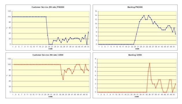
Figure 72: Fill rates and backlogs, with a supply shortage under OPT
