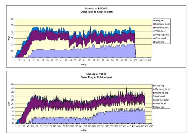
Figure 63: Lead times observed, with a supply shortage under 'pull' logistic control
