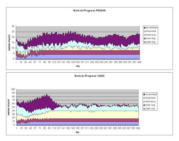
Figure 85: WIP levels observed, with a machine breakdown under OPT
