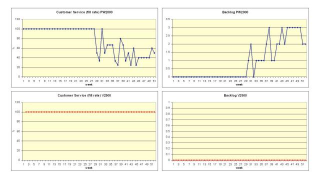
Figure 76: Fill rates and backlogs, with a machine breakdown under a 'push' system
