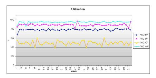
Figure 53: Observed utilisation of key workcentres, with quality problems in a 'push' system
