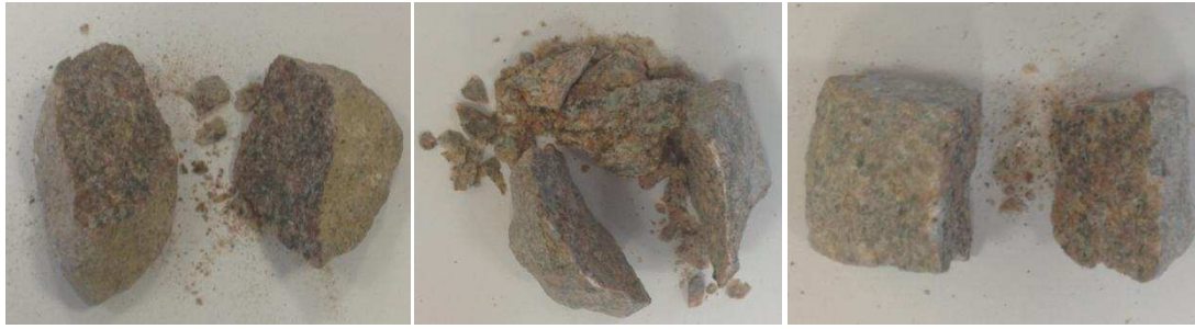
Figure 8 Photographs showing the typical daughter fragments produced following the failure of the single parent particles subjected to a diametrical compression test
