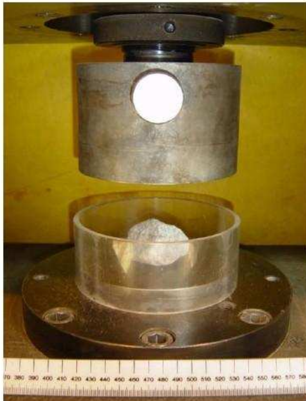
Figure 5 A photograph of the Zwick experimental testing rig used to apply diametrical compression tests to selected rock samples.
