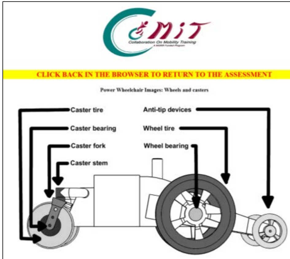
Figure 8. Example of illustration used to indicate wheelchair components mentioned in the self-reported repairs questionnaire.
