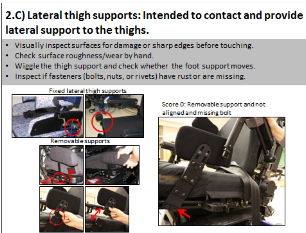
Figure 6. Example of an item description in the PW-MAT V2 illustrated guide used during the round of reliability testing.
