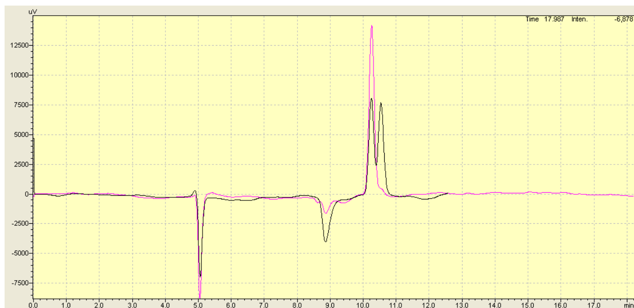
Figure 3.10 HPLC traces for conjugate addition product of 3.29: Enantioenriched sample (pink) and racemic mixture (black)
