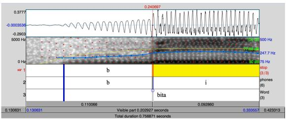
Figure 3: Example of Segmentation
