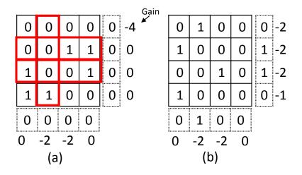
Figure 13: An example of CAFO's optimization. A data cell with "0" represents a match with the already written bit, "1" otherwise. The cost of flipping an intersecting matching cell  $c_{r,c}$  is -1. Flipped rows and column are highlighted in red. The number of bit flips is reduced from 6 to 4.
