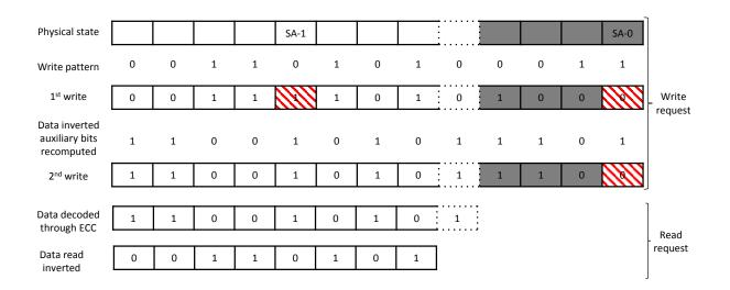
Figure 22: An example of executing write and read requests with integrated protection complementing an error correcting code of capability 1. Dotted cells represent the polarity bit, grey cells represent the auxiliary bits and red patterned cells represent errors.
