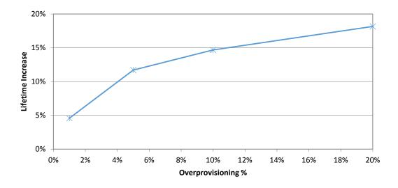
Figure 39: Lifetime increase achieved by data dependent sparing at various levels of over-provisioning compared with static sparing with 20% over-provisioning.
