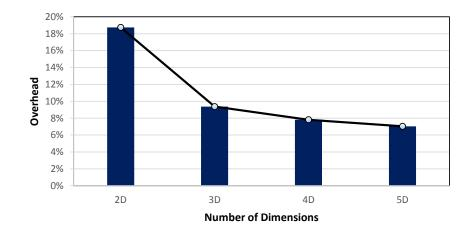
Figure 31: Space overhead of RDIS for a 512-bit block with various dimensional arrangements.
