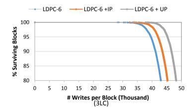
Figure 48: Lifetime of PCM main memory blocks achieved with LDPC-6 and LDPC-6 complemented by Symbol Shifting with integrated protection (IP) and un-integrated protection (UP).
