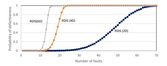
Figure 34: Probability of defectiveness with different dimensional arrangements for a 4096-bit block.
