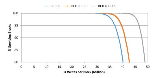
Figure 26: Lifetime of PCM main memory blocks achieved with BCH-6 and BCH-6 complemented by data inversion with integrated protection (IP) and un-integrated protection (UP).
