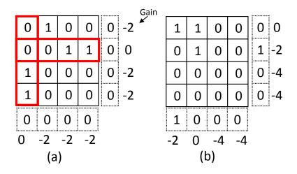
Figure 12: An example that shows that the cost of a write can still be reduced even when no row or column shows a positive gain. A data cell with "0" represents a match with the already written bit, "1" otherwise. Flipped rows and column are highlighted. The number of bit flips is reduced from 5 to 3.
