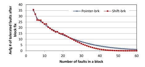
Figure 32: Avg. number of additional tolerated faults after breaking a defective pattern in a 2048-bits block size.
