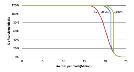
Figure 41: Lifetime of PCM blocks under two failure frequency threshold values: 5% vs. 10%. "DD" denotes data dependent sparing and "SS" static sparing.
