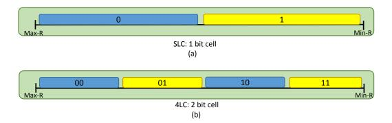
Figure 5: The concept of multilevel PCM cell.
