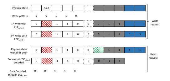
Figure 47: An example of encoding/decoding with Composite Capability. Dotted Cell represents the SSC. Grey cells represent  $ECC_{hard}$  auxiliary bits. Blue cell represents  $ECC_{drift}$  auxiliary bits. Red diagonal patterned cells represent stuck-at cell errors. Green brick patterned cells represent drift errors.
