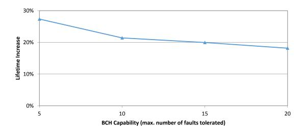
Figure 40: Lifetime increase achieved by data dependent sparing relative to static sparing for various BCH code capabilities.
