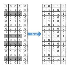
Figure 11: An example of Flip-N-Write (FNW) encoding where the number of bit flips is reduced from 33 to 25. A data cell with "0" represents a match with the already written bit, "1" otherwise. Shaded cells represent a row that is to be flipped.
