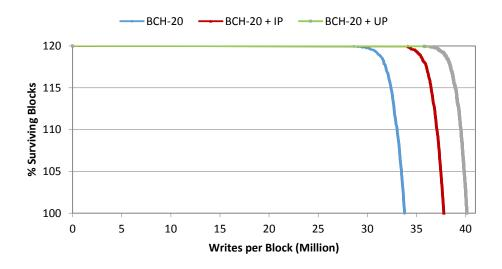
Figure 27: Lifetime of PCM storage blocks achieved with BCH-20 and BCH-20 with integrated protection (IP) and un-integrated protection (UP). This experiment assumed that 20% of spare storage capacity was provided.
