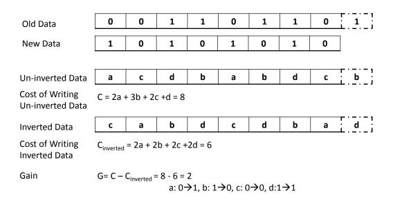
Figure 14: An example of taking the cost of the auxiliary bit into consideration when computing the gain. The costs of "a", "b", "c" and "d" are 1, 2, 0 and 0 respectively. Dotted cells represent auxiliary bits.
