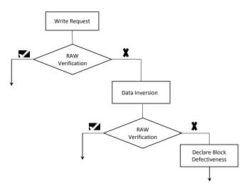
Figure 25: Flow of executing a write request. "RAW" denotes read after write.
