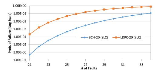
Figure 49: Probability of failing to write on 4KB SLC and 3LC blocks protected by BCH-20 and LDPC-20 respectively.
