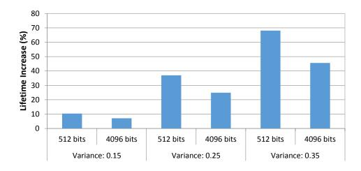
Figure 28: Lifetime increase with BCH complemented with data inversion relative to regular BCH with various cell lifetime variance.
