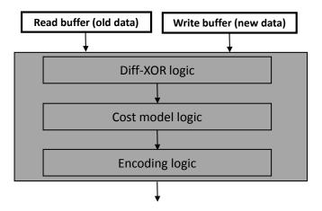
Figure 15: Write datapath logic for CAFO.
