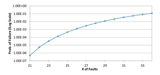
Figure 29: Probability of the first write failure on a 512-bytes storage block protected by a BCH-20 code.
