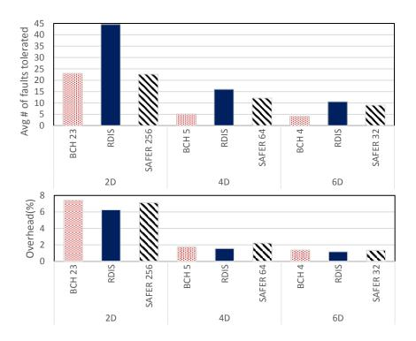
Figure 33: Average number of faults that can be tolerated by RDIS with various dimensional arrangement compare to SAFER and BCH for 4096-bit block.
