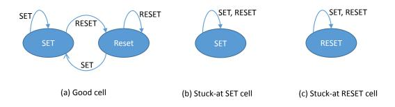
Figure 4: Difference between a good and stuck cell.
