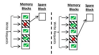
Figure 36: Data-dependent Sparing. Shaded cells represent defective blocks.
