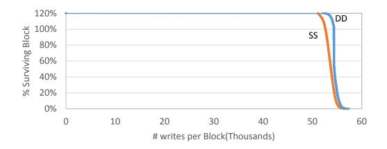
Figure 50: Lifetime Improvement with Data Dependent Sparing (DD) in the context of 3LC in comparison to Static Sparing (SS).
