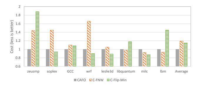
Figure 21: Cost reduction achieved by CAFO over cost aware Flip-N-Write (C-FNW) and Flip-Min (C-Flip-Min).
