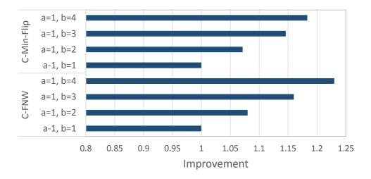
Figure 19: Cost reduction improvement of cost aware Flip-N-Write (C-FNW) and Flip-Min (C-Flip-Min) over cost oblivious Flip-N-Write and Flip-Min through the integration of CAFO's cost model.
