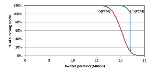
Figure 38: Lifetime of PCM blocks with BCH-20 and 10% failure frequency threshold. "DD" denotes data dependent sparing and "SS" static sparing.
