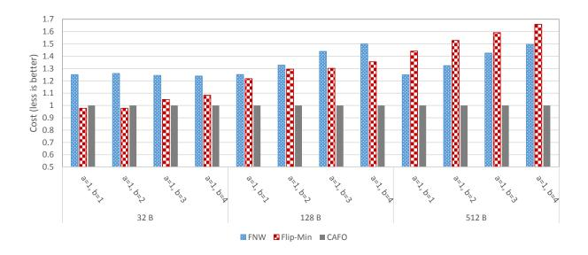
Figure 17: Cost reduction achieved by CAFO over Flip-N-Write (FNW) and Flip-Min.
