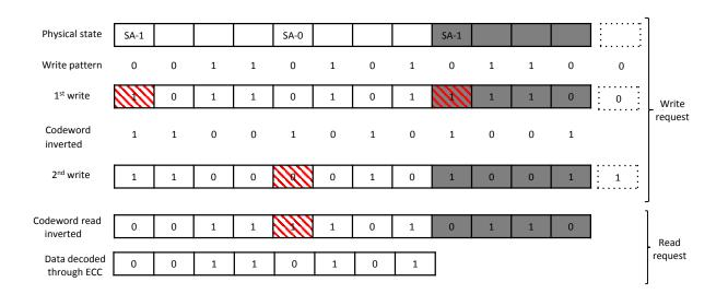
Figure 23: An example of executing write and read requests with un-integrated protection complementing an error correcting code of capability 1 protecting one byte of memory. Dotted cells represent the polarity bit, grey cells represent the auxiliary bits and red patterned cells represent errors.
