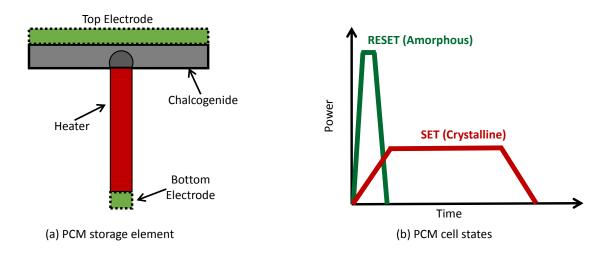
Figure 3: An example of PCM storage elements (a) and the states it can take (b).
