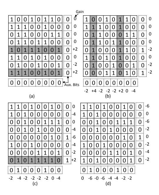
Figure 10: CAFO encoding example where the number of bit flips is reduced from 33 to 21. A "0" represents a matching cell (c = d = 0), and a "1" represents a non-matching cell (a = b = 1). "Gain" is calculated as per Formula (3.2). Shaded cells represent rows and columns that are to be flipped.
