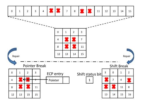
Figure 30: Defective block fixing techniques.
