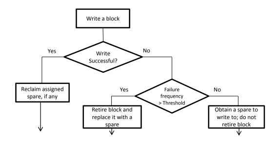
Figure 37: Flow of execution in data dependent sparing.
