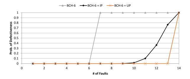
Figure 24: Probability of defectiveness as a function of the number of stuck-at faults, where a BCH-6 protects a block of size 512 bits. "IP" denotes integrated protection and "UP" denotes un-integrated protection.
