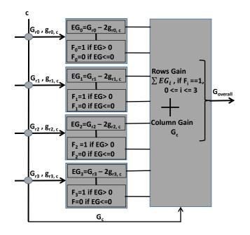
Figure 16: Optimization logic. EG is the expected gain of flipping a row. G is the initial gain of rows or columns.  $g_{r,c}$  is the gain of flipping the cell intersecting at row r and column c. F is a control signal to flag positive EG.  $G_{overall}$  is the overall gain of flipping the selected column with the rows with EG > 0.
