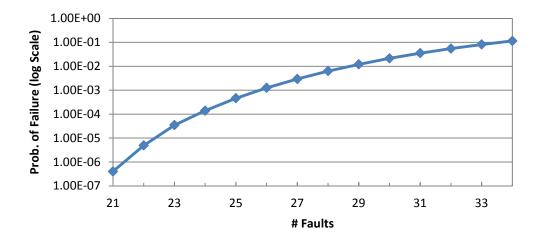
Figure 35: Block write failure probability vs. # of faults within a 4KB storage block, when an error correction mechanism covers up to 20 errors.
