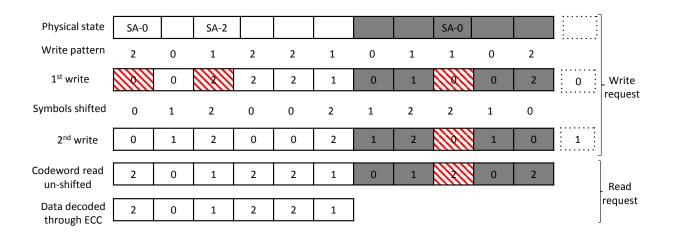
Figure 46: An example of and (6, 11) LPDC code for ternary cells of capability 2 complemented by data shifting with un-integrated protection. Dotted cells represent the SSC, grey cells represent the auxiliary cells and red patterned cells represent symbol errors.
