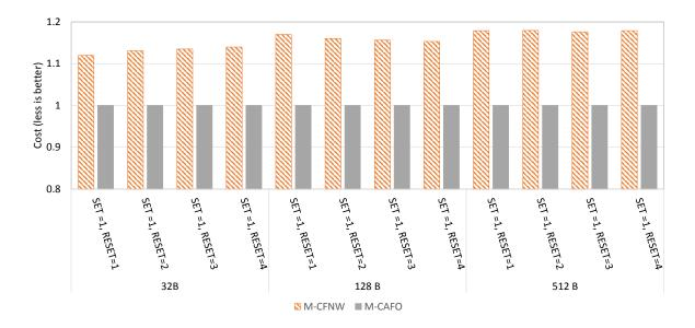
Figure 45: Cost reduction of M-CAFO over M-CFNW in the context of 3LC PCM cells.
