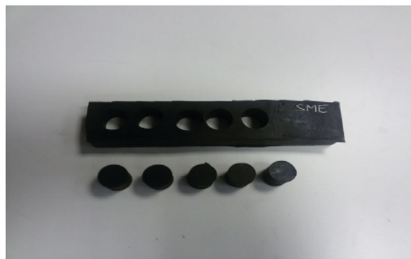
Fig. 6 The device used for rapid wear testing
