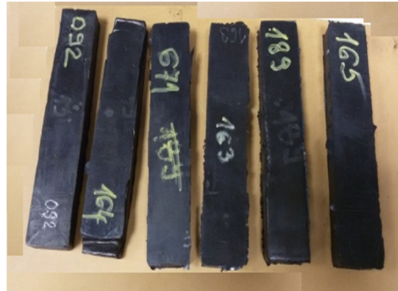
Fig. 2 Bodies for the preparation of samples for quick wear testing
