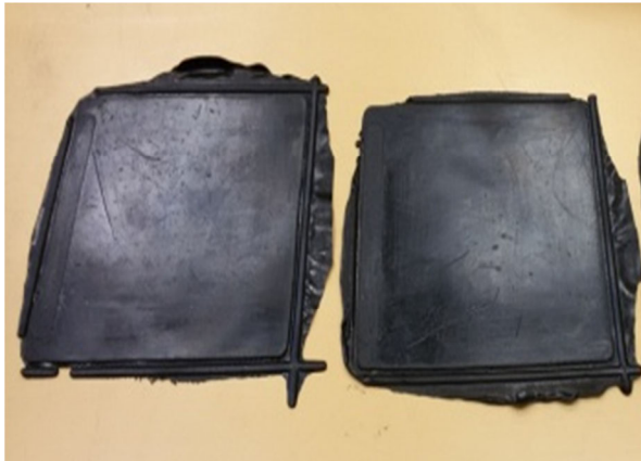
Fig. 1 Plates for the cutting of blades
