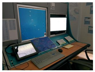
Fig. 2. The ATCO working position of the BEST Radar Simulator at the Faculty of Transport and Traffic Sciences
