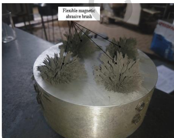
Figure 5. Formation of flexible magnetic abrasive brush
