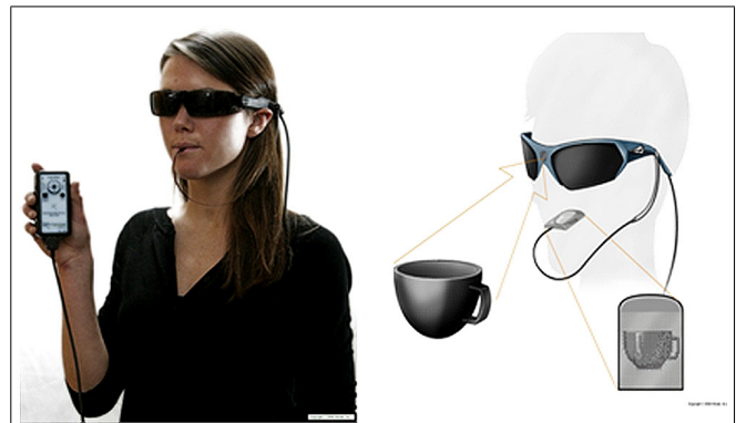
FIGURE 1 | The BrainPort Vision Device is a sensory substitution system that down samples video from a glasses-mounted frame camera to a 400 pixel (20 × 20) electro tactile array. Users are able to interpret their environment by feeling the stimuli on the surface of their tongue (Courtesy, Wicab, Inc.).
