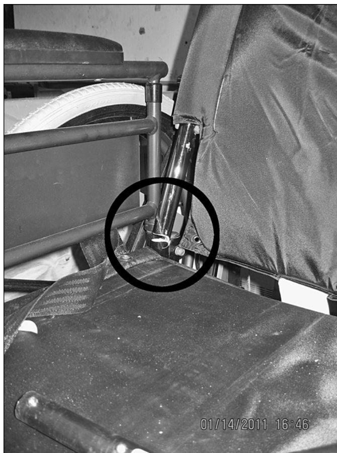
Figure 8. Invacare Patriot Plus seat upright failure.
