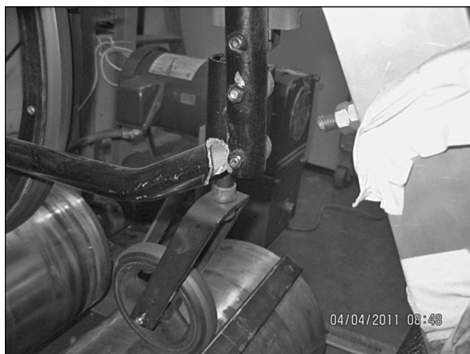
Figure 7. Failure of front-left main frame on Sunrise Medical Breezy 600 wheelchair.
