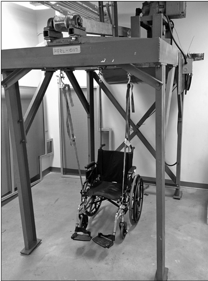
Figure 5. Curb-drop test machine (test dummy not shown).
