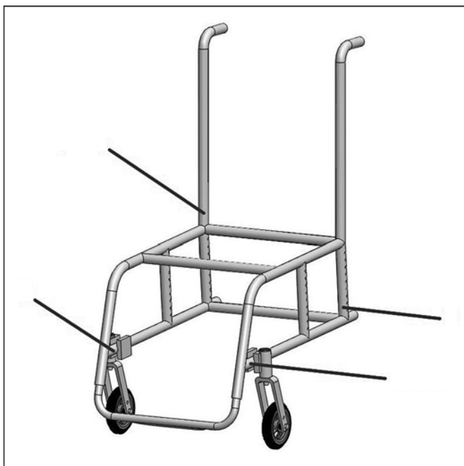
Figure 10. Locations of critical failures on wheelchairs in this study. (Rear wheels and seating system not shown.)
