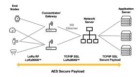
Fig. 1. A general LoRaWAN architecture according to [8].
