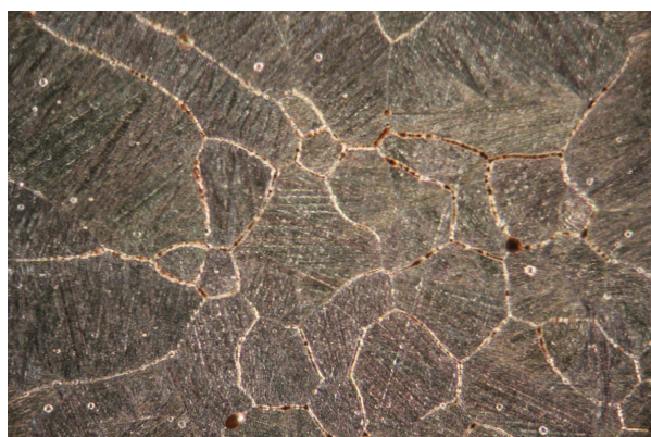
Fig. 5 – Cu-Al-Ni alloy surface after polarization measurements in 0.5 mol dm -3 H 2 SO 4 at 20 °C
