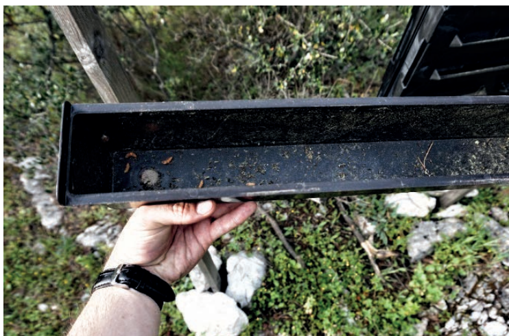
Slika 5. Suha lovna posudica feromonske klopke Figure 5 Dry catching vessel of pheromone trap
