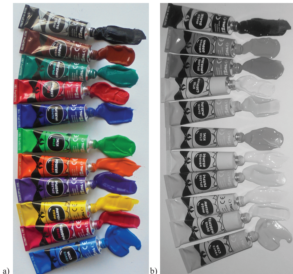
Figure 1 a) Tempera colorants for fine art paintings; b) NIR image of tempera colorants for measurement of Z value at 1000 nm
