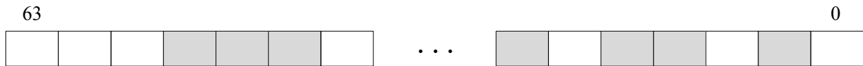
(a) A memory slice is divided into 64 B-blocks. 32 B-blocks (grey) are selected to construct a superpage.
