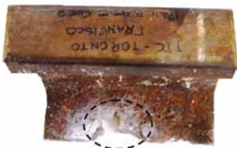
Figure 9. Tested sample of corroded rail, loss of material from the side and top part of the rail foot: circled points are the points of concentration of highest normal stresses [31]
