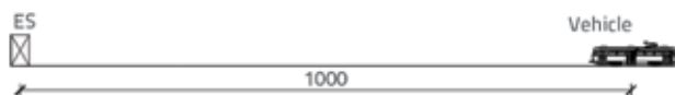
Figure 14. Schematic of the observed track segment, vehicle 1000 m away from the electrical substation (ES)
