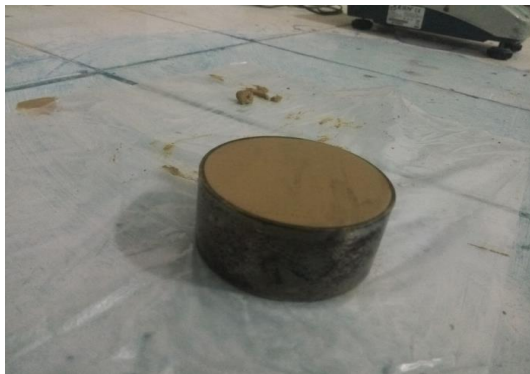
Figure 3 Compacted sample in the mold
