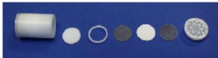
Figure 1. Ogawa sampler components
