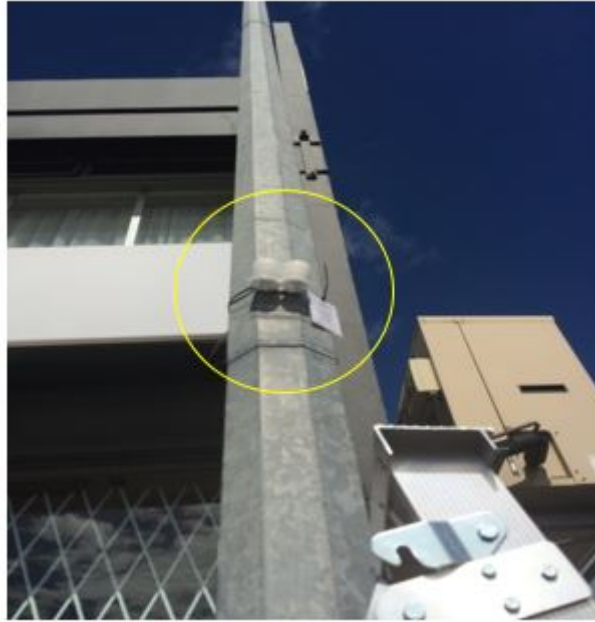
Figure 3. Gas samplers housed in Ogawa shelters
