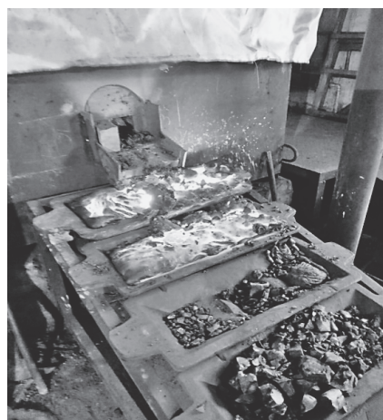
Figure 1 300 kVA furnace directly after tapping
