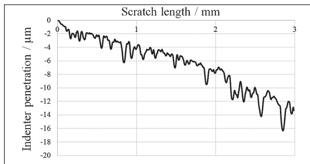
Figure 13 Indenter penetration depth versus scratch length in a-C:H
