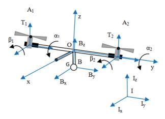
Figure 2. Modelling diagram of the tandem tilt-rotor.
