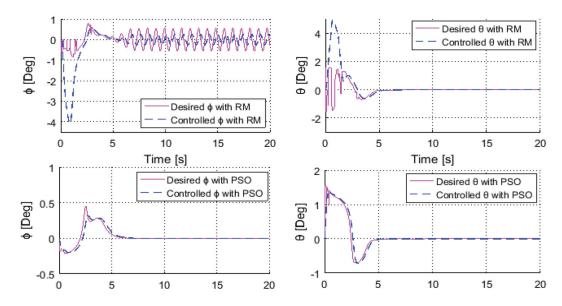
**Figure 5.** Desired and controlled roll and pitch angles  $(\phi, \theta)$  by using RM and PSO (first trajectory).
