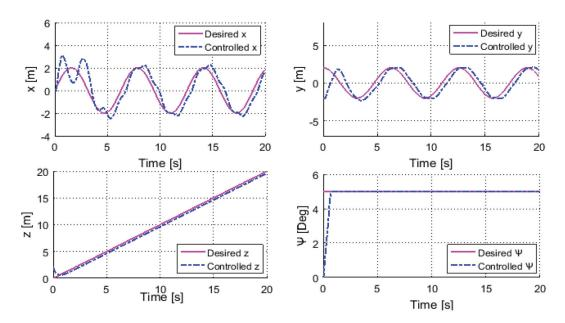
**Figure 11.** Desired and controlled position, altitude and yaw angle  $(x, y, z, \psi)$  by using PSO in presence of external disturbances (second trajectory).
