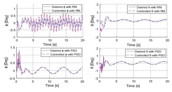
**Figure 8.** Desired and controlled roll and pitch angles  $(\phi, \theta)$  by using RM and PSO (second trajectory).
