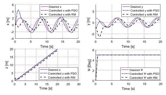
**Figure 7.** Desired and controlled position, altitude and yaw angle  $(x, y, z, \psi)$  by using RM and PSO (second trajectory).
