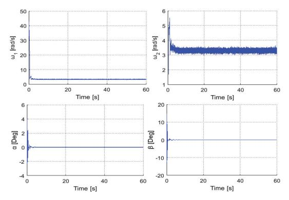
**Figure 19.** Rotors' angular speeds ( $\omega_1$  and  $\omega_2$ ) and tilting angles ( $\alpha$  and  $\beta$ ).
