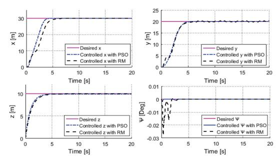
**Figure 4.** Desired and controlled position, altitude and yaw angle  $(x, y, z, \psi)$  by using RM and PSO (first trajectory).
