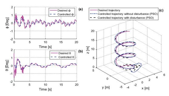
**Figure 12.** Desired and controlled PSO responses in presence of external disturbances for roll  $\phi$  (a) and pitch  $\theta$  (b) angles; (c) desired and controlled PSO trajectories without/with presence of disturbances in 3D (second trajectory).
