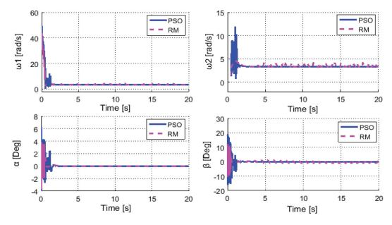
**Figure 9.** Rotors' angular speeds ( $\omega_1$  and  $\omega_2$ ) and tilting angles ( $\alpha$  and  $\beta$ ) (second trajectory).
