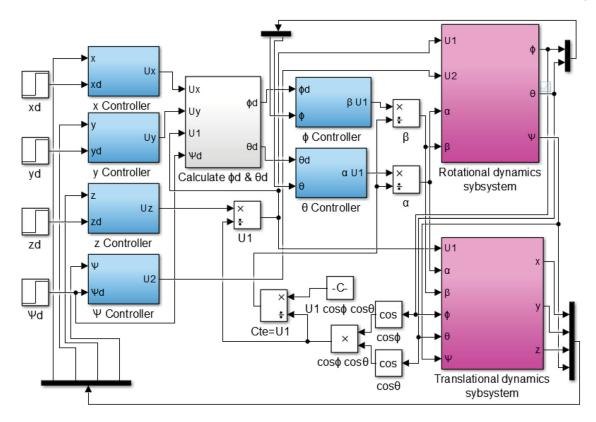
Figure 3. Tilt-rotor's control loop.
