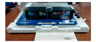
**Figure 11.** Motor-generator coupling to analyse load-torque variations.
