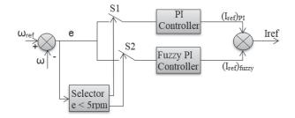
Figure 10. Structure of hybrid fuzzy PI controller.
