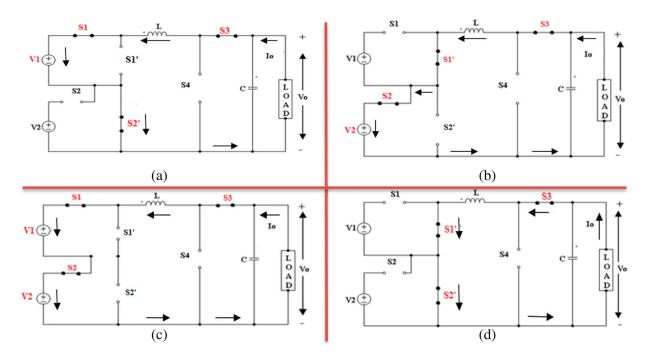
**Figure 7.** Bidirectional modes of operation (a) Individual charging of source 1 alone; (b) Individual charging of source 2 alone; (c) Simultaneous charging of energy sources 1 and 2; (d) Freewheeling of load current.
