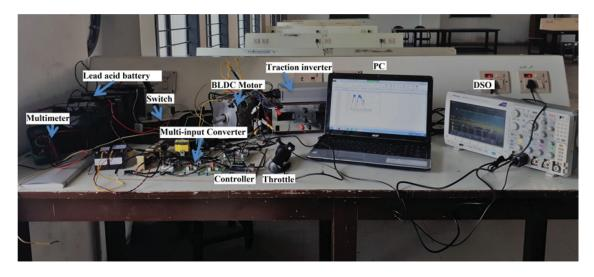
Figure 16. Experimental setup.
