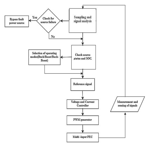
Figure 8. Control signals generating scheme for multi-input Converter.
