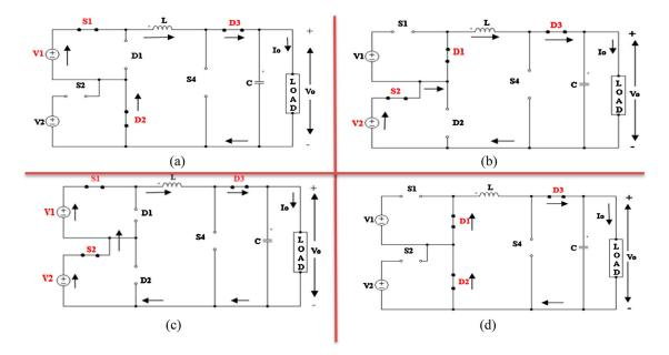
**Figure 5.** Various possible working states (a) Individual utilization of voltage source V1; (b) Individual utilization of voltage source V2; (c) Simultaneous utilization of V1 and V2; (d) Freewheeling of load current.
