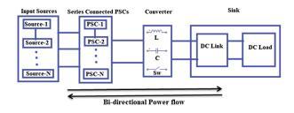
Figure 3. Architecture of multi-input converter.
