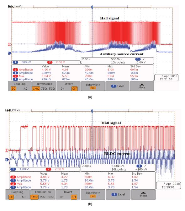
Figure 20. (a) Hall signals during acceleration; (b) Hall signal and stator current of BLDC Motor during acceleration.
