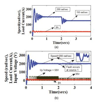
**Figure 12.** (a) Speed regulation for step change and the armature current waveform; (b) Speed regulation under healthy and faulty condition of source.
