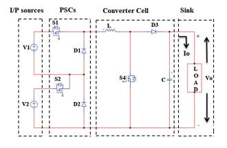
Figure 4. Multi-input converter system with two input sources.
