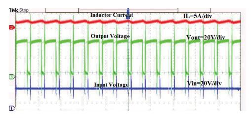
**Figure 17.** The inductor current, output voltage and input voltage of the MIC with  $R = 10 \Omega$ .
