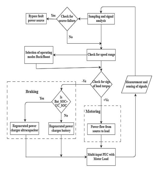
Figure 9. Power management algorithm for bi-directional power flow.
