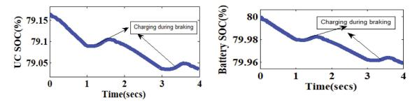
Figure 15. Charging and discharging of UC and battery during various operation of speed profile.
