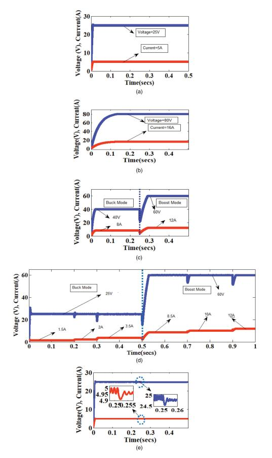
**Figure 11.** (a) Output voltage and load current waveforms for buck mode; (b) Output voltage and load current waveforms for boost mode; (c) Step change in output voltage during buck and boost mode; (d) Voltage and current waveform for buck and boost mode during different loading condition; (e) Regulation of voltage under the faulty condition.
