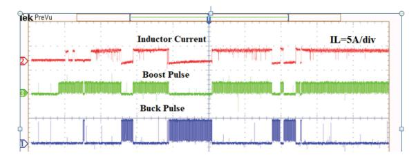
Figure 19. Inductor current, boost and buck pulse waveform for acceleration and constant speed operation.
