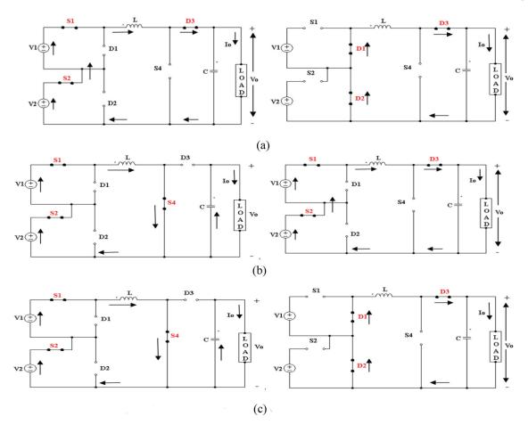
**Figure 6.** Various operating modes (a) Circuit configuration during buck mode of operation; (b) Circuit configuration during boost mode of operation; (c) Circuit configuration during buck-boost mode of operation.
