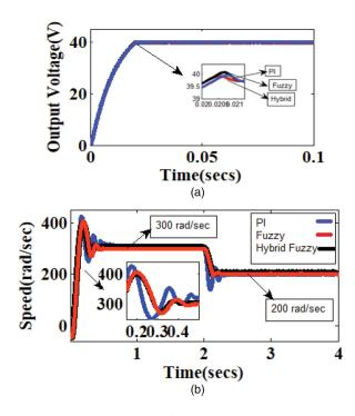
**Figure 13.** (a) Comparison of PI, fuzzy and hybrid Fuzzy PI controller for voltage regulation; (b) Comparison of PI, fuzzy and hybrid fuzzy PI controller for speed regulation.
