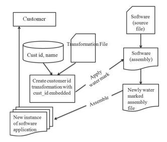
Figure 1. System architecture-watermarked code.
