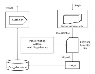
Figure 2. Flow of providing security-disassemble system.
