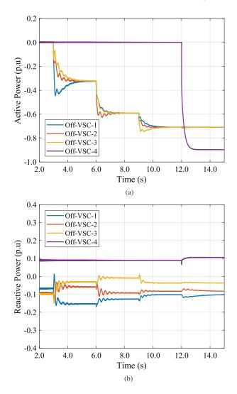
**Figure 9.** The power response of offshore VSCs. (a) Active power response and (b) reactive power response.
