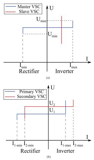
**Figure 2.** The characteristic curve of master–slave and voltage margin control principle. (a) Master-slave principle and (b) voltage margin principle
