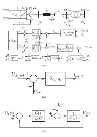
**Figure 6.** Onshore VSC substation and its control scheme for MTDC network. (a) Onshore VSC Control, (b) DC voltage control with proportional regulator, and (c) stability model of DC voltage with proportional regulator
