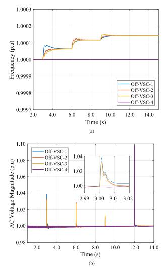
**Figure 10.** The response of offshore VSCs frequencies and their corresponding busbar voltages. (a) Frequencies imposed by offshore VSCs and (b) AC voltages at VSCs busbars.
