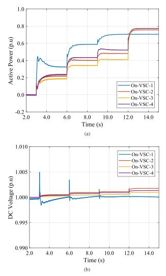
**Figure 11.** The active power and DC voltage response of the onshore converters. (a) Active response and (b) DC voltages at VSCs busbars.
