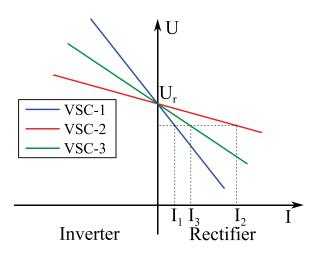
**Figure 7.** *U–I* characteristic of onshore VSCs DC voltage control to operate MTDC network.
