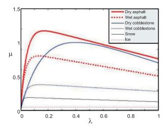
**Figure 2.** The variation of the friction coefficient,  $\mu$  against the slip ratio,  $\lambda$  on different road conditions [1].
