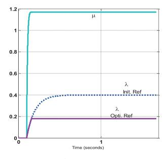
**Figure 6.** The ABS performance using  $\mu$  peak detector and the optimal slip ratio reference.
