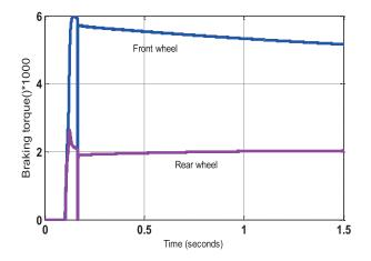
Figure 9. The rear and front wheels braking torques.
