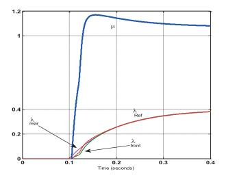
**Figure 5.** The ABS controller performance in tracking the issued arbitrary slip ratio command.
