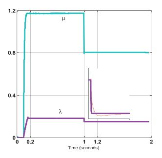
**Figure 11.** Effective braking on a nonuniform road condition; the varying optimal reference slip ratio reference ( $\lambda$ ) and the maximum attainable tire-road friction coefficient ( $\mu$ ).
