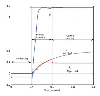
Figure 4. The braking timing.
