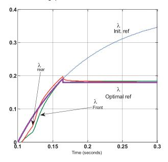
**Figure 8.** The performance of the ABS adaptive sliding mode control using  $\hat{v}$ .
