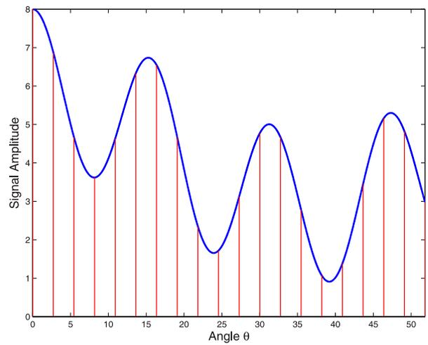
**Figure 2.** Data sampling in angular domain.
