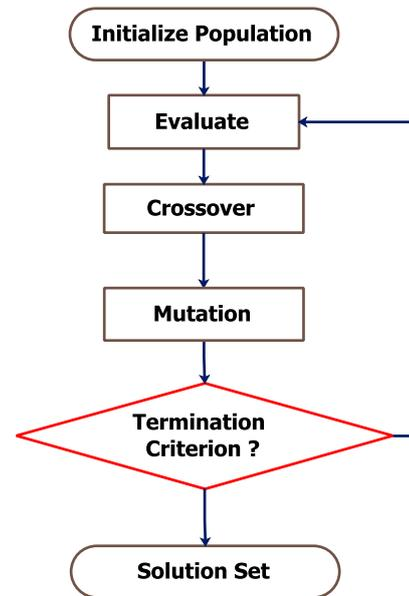
**Figure 4.** Genetic algorithm diagram.
