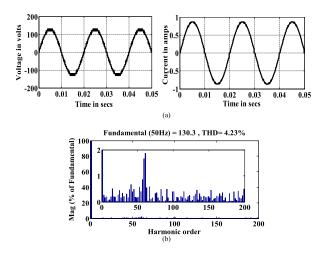
Figure 3. Output voltage and current with FFT Plot for PDPWM scheme.
