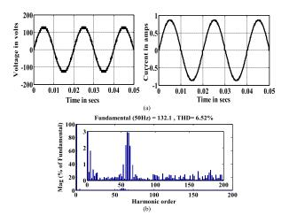
**Figure 5.** Output voltage and current with FFT plot for CO PWM Scheme.
