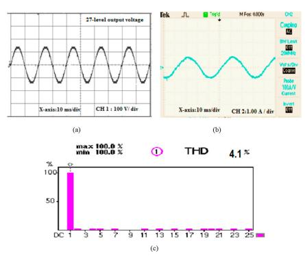
Figure 9. Experimental results: (a) output voltage, (b) output current, and (c) voltage FFT Plot for PD PWM type.
