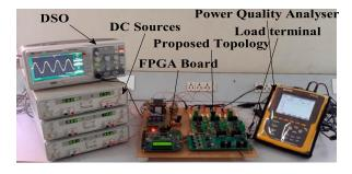
**Figure 7.** Prototype model of proposed 27 level single phase trinary DC source CMLI.
