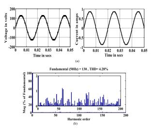
**Figure 6.** Output voltage and current with FFT Plot for VF PWM scheme.
