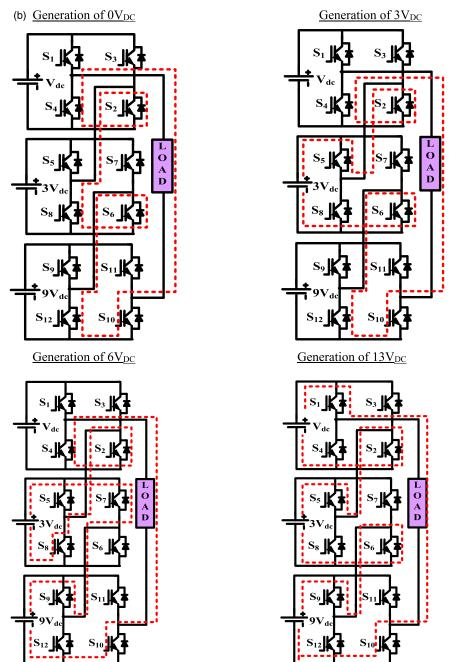
Figure 1. (a) Proposed trinary DC source multilevel inverter. (b) Sample modes of operation of proposed trinary MLI for positive polarity generation.
