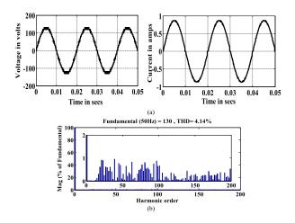
**Figure 4.** Output voltage and current with FFT plot for APOD-PWM Scheme.
