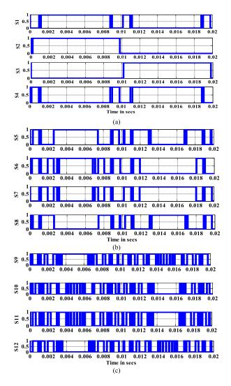
**Figure 8.** Switching signals for the proposed topology. (a) Switching signal for first bridge, (b) switching signal for second bridge, and (c) switching signal for third bridge.
