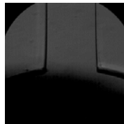
Figure F. 36. Left and right walls of the inlet region of a representative serpentine microchannel filled with 1% bovine serum albumin. 40x magnification. Field of view in each image is 500 \mu\text{m} by 500 \mu\text{m} .
