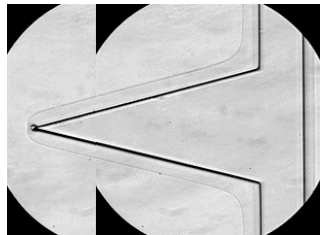
Figure F. 10. Fourth crevice in the flow path of the Crevice microchannels prior to sealing. 40x magnification.
