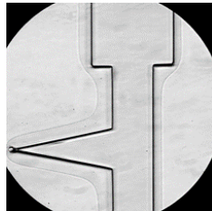
Figure F. 14. Eighth crevice in the flow path of the Crevice microchannels prior to sealing. 40x magnification. Field
