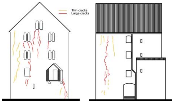
Fig. 8 Crack pattern investigation of the Pišce Castle (courtesy of Politecnico di Milano)
