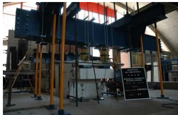
Fig. 2 System of load application
