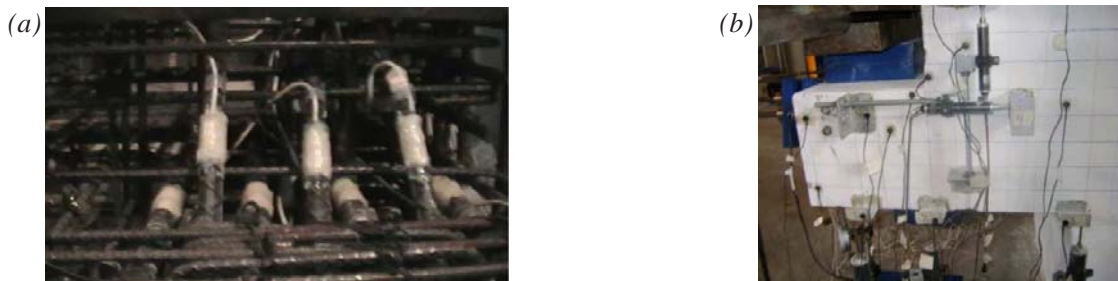
Fig. 3 Instrumentation of steel bars and external instrumentation: (a) placement of strain gauges; and (b) placement of potentiometers
