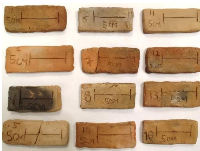
Figure 42: Experimental tiles after firing
